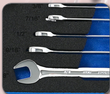
Laser cut "tight fit" tool cutouts.
